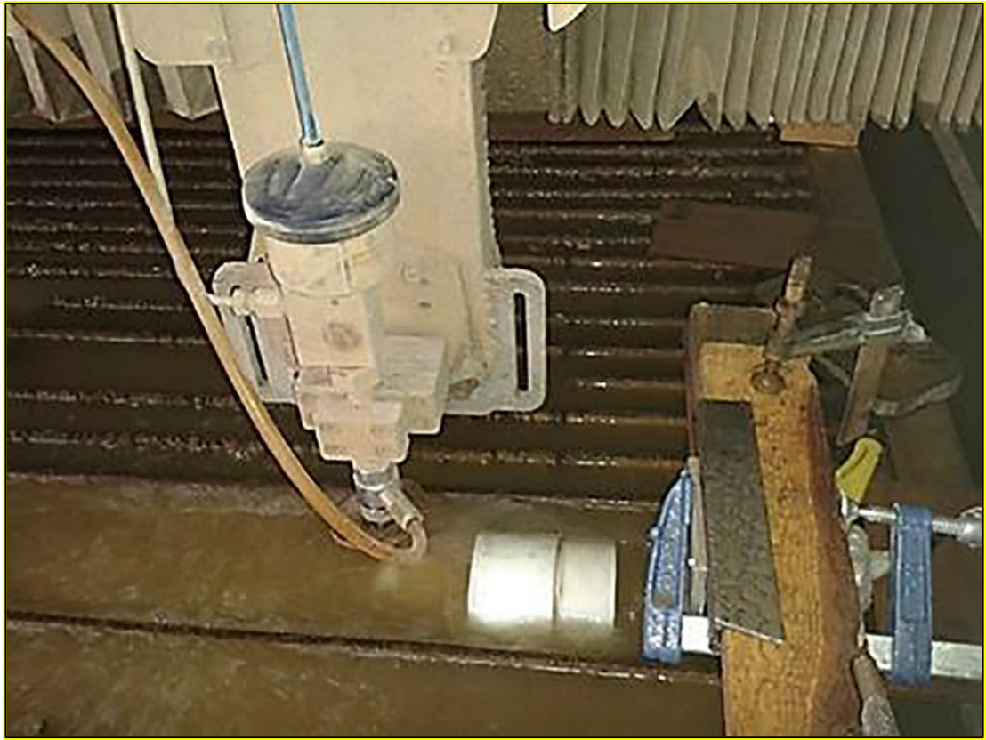
Figure 5.3. Submerged abrasive water jet experimental setup.
