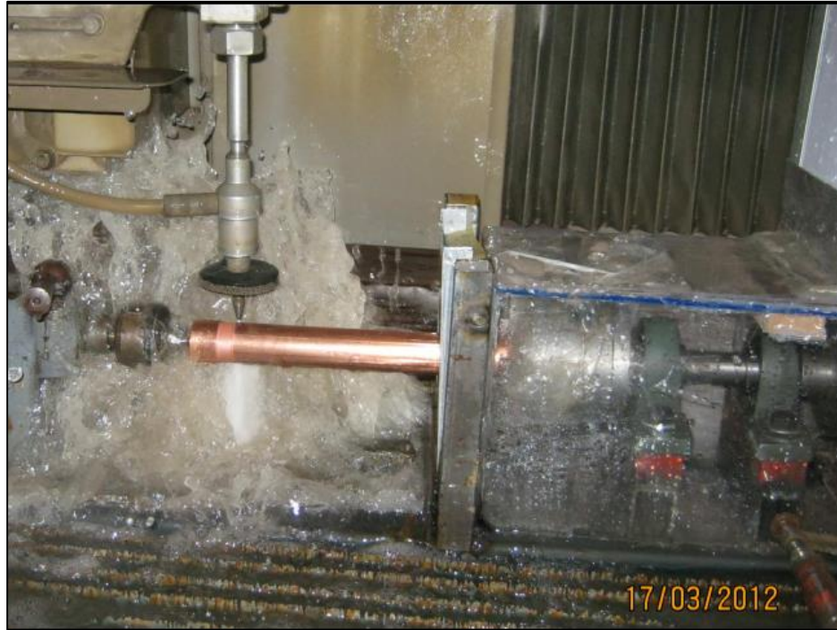
Figure 2.12. Grinding disk during experimental turning [39].
