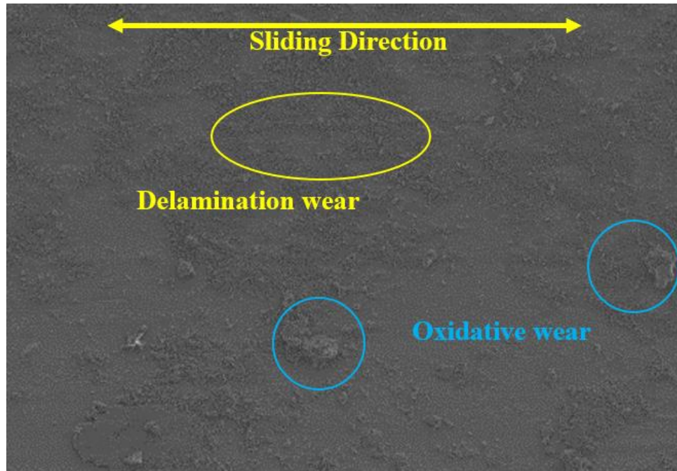
Figure 4.8. FESEM images of heat-treated specimens at x500 for B1 (Layer thickness: B1=11.0 \mu\text{m} ).
