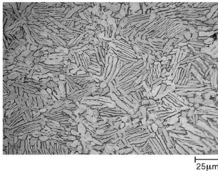
Figure 2.24. Casting Widmanstatten structure with \alpha -phase in light color and \beta -phase is dark color [61].
