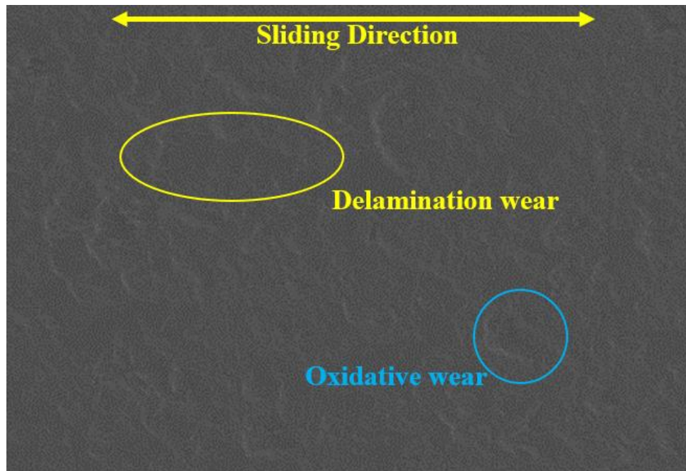
Figure 4.9. FESEM images of heat-treated specimens at x500 for B2 (Layer thickness: B2= 10.4 \mu\text{m} ).
