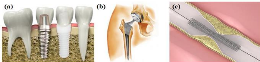
Figure 2.16. Application of titanium alloys in the biomedical; (a) dental implant [47], (b) hip joint, (c) vascular stent [48].
