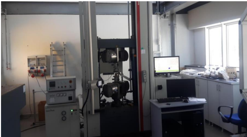
Figure 3.7. Zwick/Roell Z600 universal test machine.
