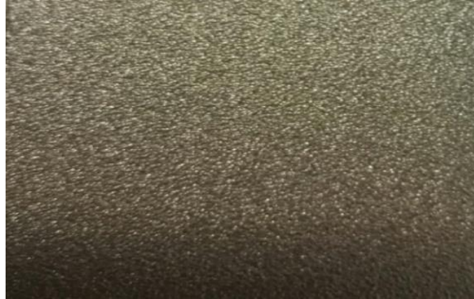
Figure 3.5. Surface of ST37-2 after shot peening; A28-30.
