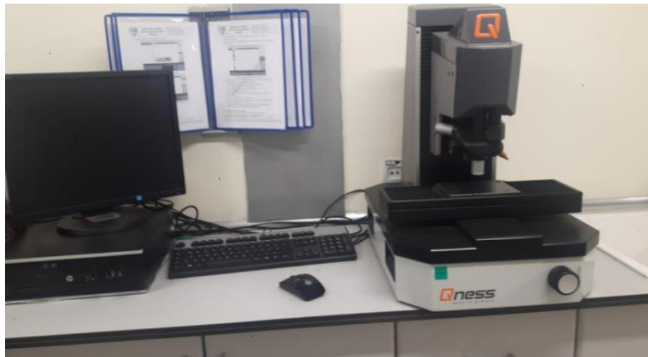
Figure 3.8. Q10 A+ QNESS microhardness testing machine.
