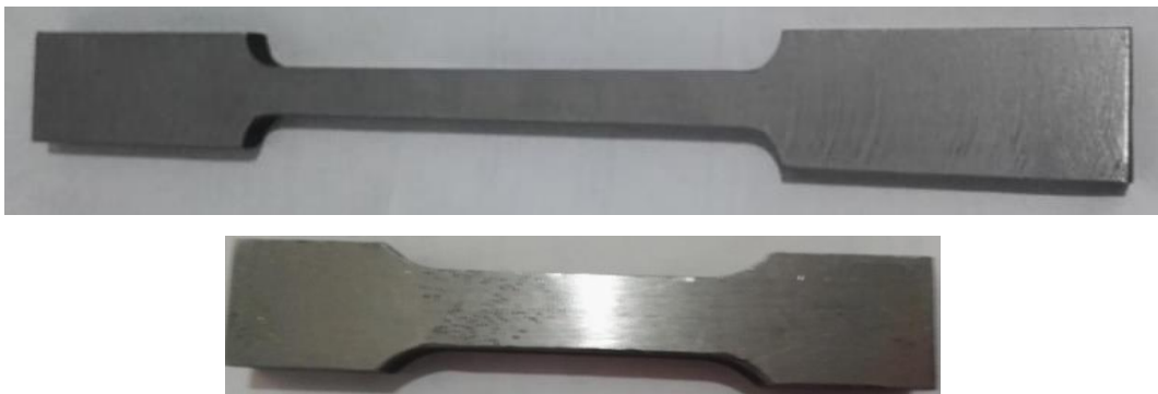
Figure 3.3. Samples for tensile testing (top) and fatigue testing (bottom).
